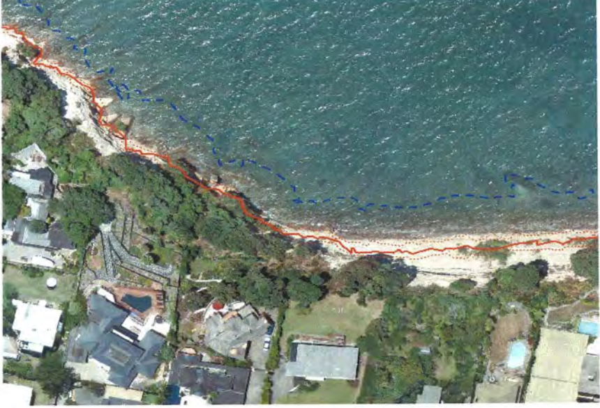
LiDAR output showing MSL (blue line) and MSL + 1.5 m (red line). Dotted red line shows +/- 0.5 m of the red line. Aerial photography (2008)
