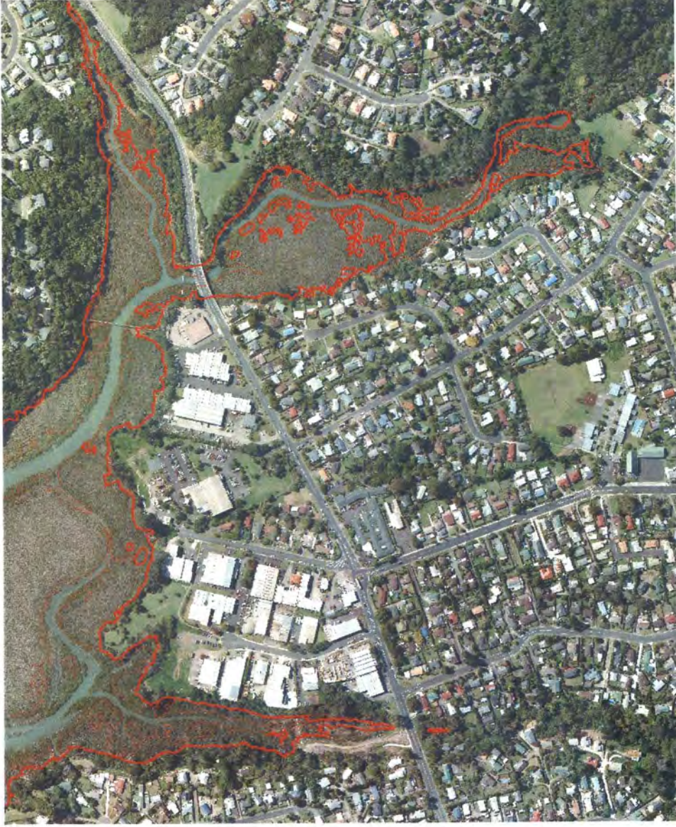
Example of LiDAR applied to a complex estuary receiving input from three tributary streams. LiDAR river mouth extents closely match coastal plan Schedule 7 CMA boundaries for all three tributaries.
