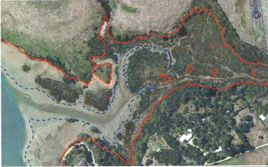
LiDAR output showing MSL (blue line) and MSL + 1.5 m (red line). Dotted red line shows +/- 0.5 m of the red line. Aerial photography (2008)
